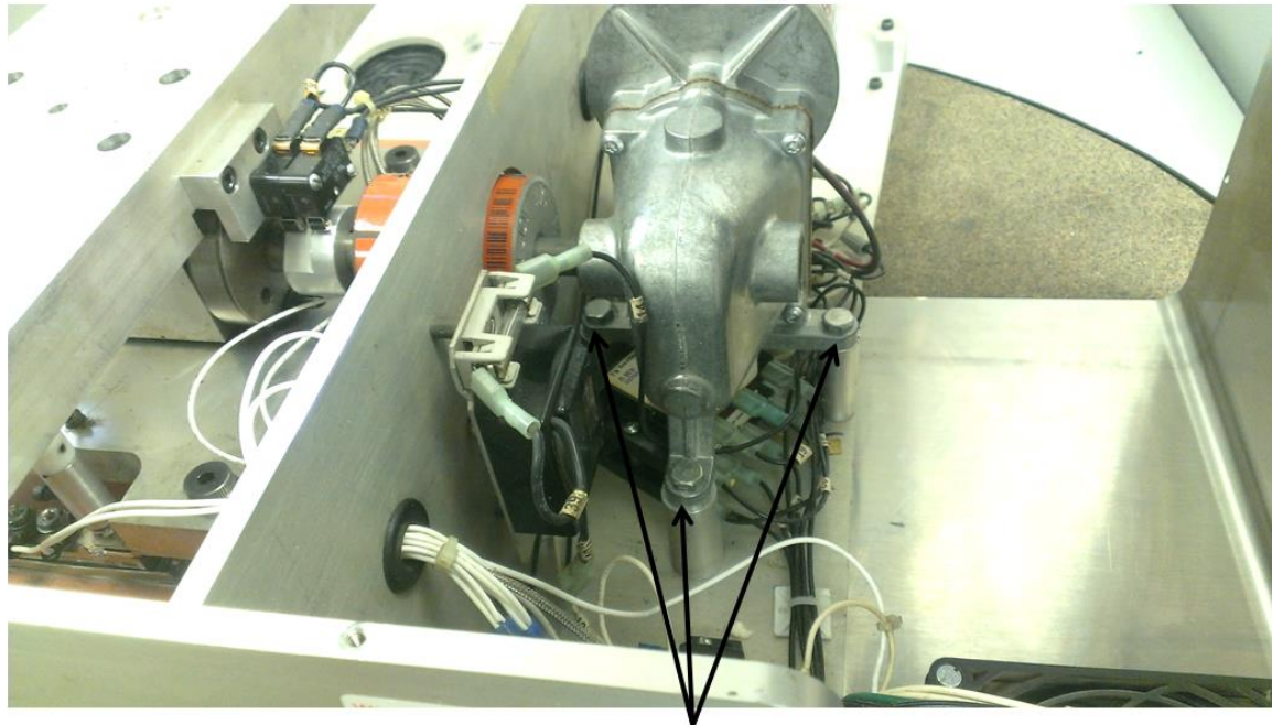
Motor Mounting Bolts 7/16" Socket Wrench
