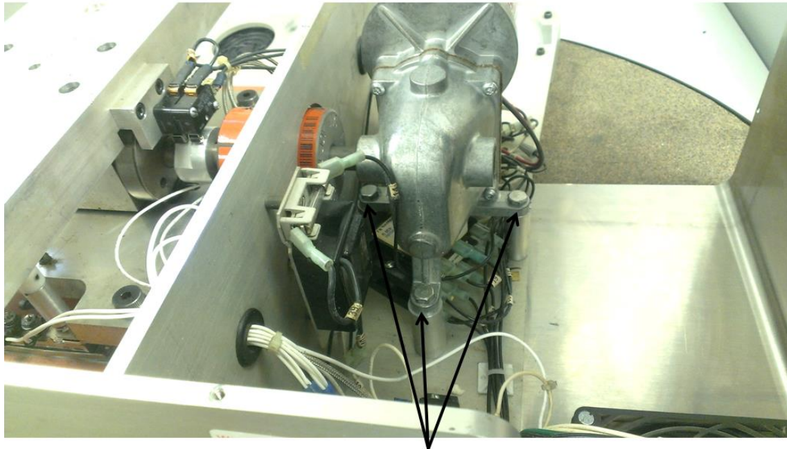
Motor Mounting Bolts 7/16" Socket Wrench
